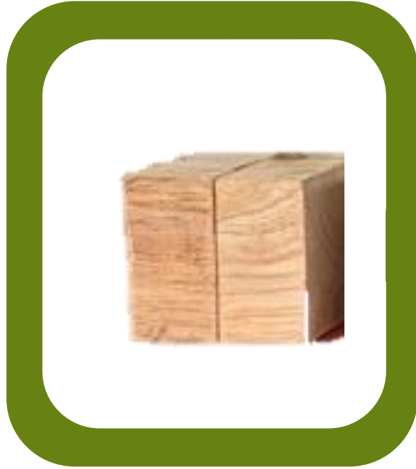
Sterilised rubber woodblock (RWB) (6x6x6 cm) inoculated with Ganoderma and incubated 8 weeks in the dark at room temperature
