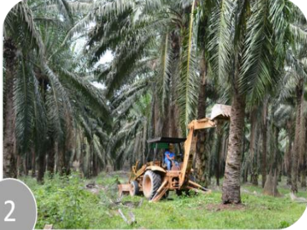
Pushing of palm with an excavator with a special cutler bucket
