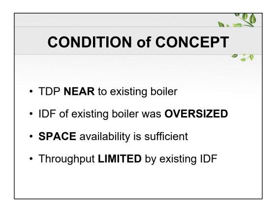
Since the TDP in Pilot Plant was couple with existing boiler, there are some limitations in scaling up of this concept:
