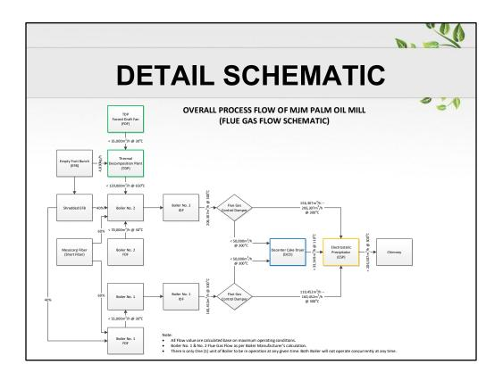
Hot flue gas from TDP channeled into Boiler may help to reduce the need of burning PKS in the boiler.
