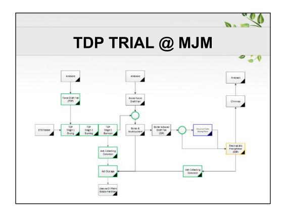
We had completed a Pilot Plant in MJM Palm Oil Mill by retrofitting the current Boiler set up to incorporate TDP into the overall process flow. Basically, we added a high efficiency combustion chamber that is able to burn 100% EFB couple with the current boiler operation mainly for EFB disposal. From the Pilot Plant, we found that the Ash generated consist of 25-30% potassium content which can be used as fertilizer.
