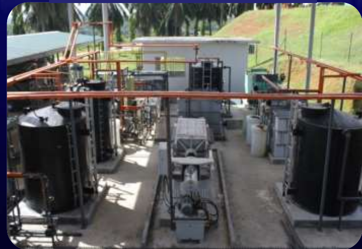
4) Loji rintis DAF dan kitar semula air (DAF and water recycling system)
