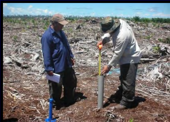
Measuring groundwater table
